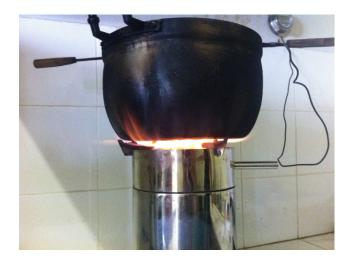
10.2. In this case we conducted the AWBT with the Philips stove, and used similar fuel (500 grams of wood pellets).
